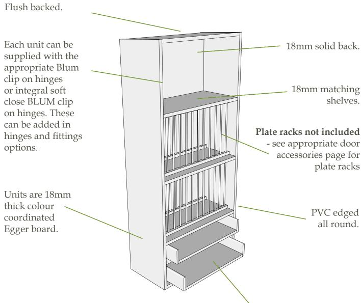
BLUM Antaro drawer box system (where drawers are included) with soft close runners, steel sides and 16mm MFC base and back. Drawers are 270mm deep and have a weight capacity of 30kg up to 800mm wide and 50kg over 800mm wide.
