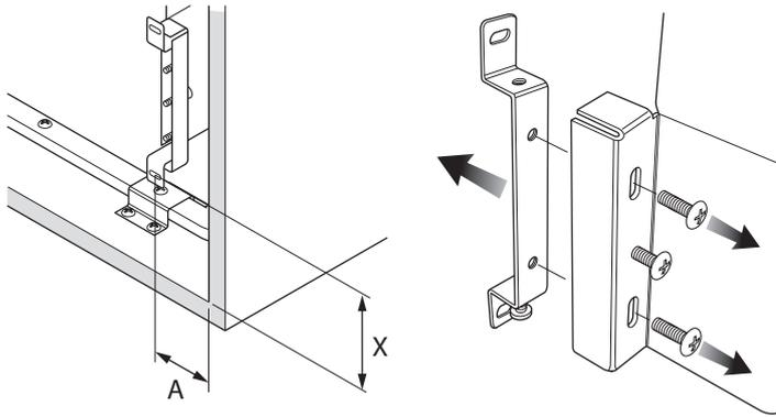
Measure from the door bracket to the cabinet base (X). Measure from the door bracket to the cabinet inside (A).
