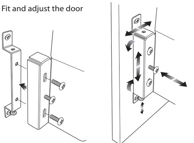
Reattach the inner brackets to the door brackets
