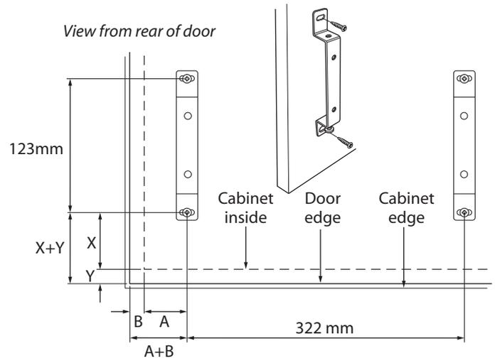
Fit the detached brackets to the door using the vertical measurements X+Y and the horizontal measurements A+B to locate. *Note: The door may not be flush with the cabinet edges.*
