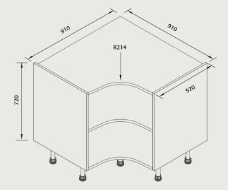
Supplied flatpack with cam & dowel fittings Can be cut down to 900 x 900 x 560D and screwed together
