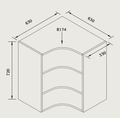
Supplied flatpack with cam & dowel fittings Can be cut down to 600 x 600 x 300D and screwed together
